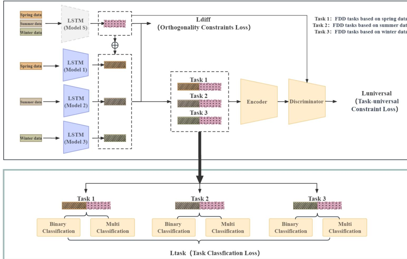
Fig. 3. Diagram of the proposed AML-FDD framework. At the Adversarial Multi-task Learning (AML) stage, adversarial training and orthogonality constraints are incorporated to learn the task-specific and task-shared features; the learned features are utilized for FDD classification tasks at the Fault Detection and Diagnosis (FDD) stage.
