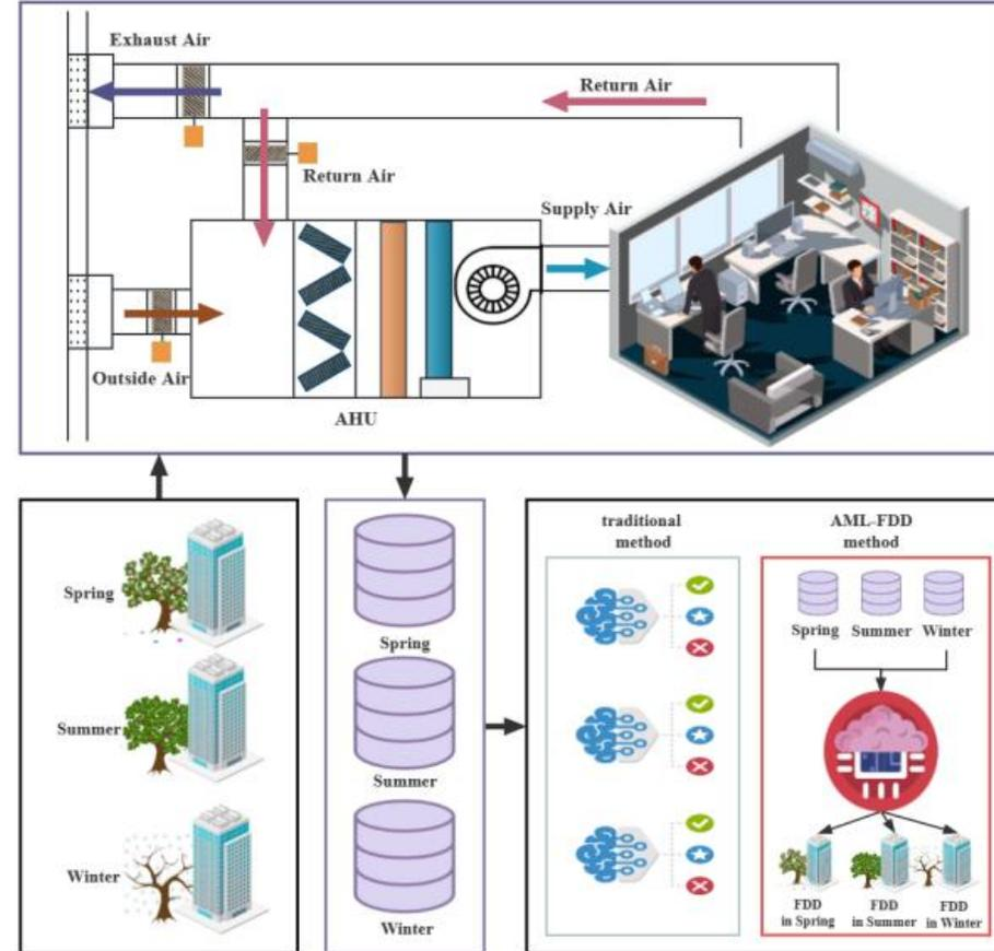
Fig. 1. An illustration of dealing with the building FDD in different ways: Single-task v.s. Multi-task.
