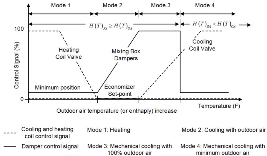
Fig. 2. Operating modes of AHU. An economizer set point refers to a predefined condition based on outdoor temperature, a combination of outdoor temperature and humidity, or outdoor enthalpy. When the outdoor temperature (and humidity) exceeds the economizer set point, the outdoor air intake will be limited to the minimum required to meet ventilation standards.
